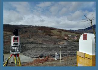
Application of advanced technologies and methods for the management of geo-hydrological disasters for civil protection purposes. Application of innovative monitoring techniques, such as radar and laser portable devices, in order to assess slope and ground deformations. Design and implementation of **Early Warning Systems.**
